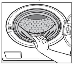
Check the folds in the door seal for any small articles, e.g. buttons. Remove any fluff from drying from around the door seal.
