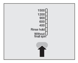
Press the "Spin" button repeatedly until the indicator lamp for the spin speed you want for the thermospin comes on.
