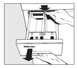
■ Pull out the detergent dispenser drawer until a resistance is felt. Press down the red release catch and at the same time pull the drawer right out of the machine.
