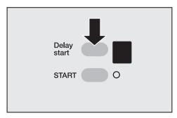
■ Press the *Delay start* button repeatedly until the required delay start period shows up in the display (from *I* to *9* hours).
