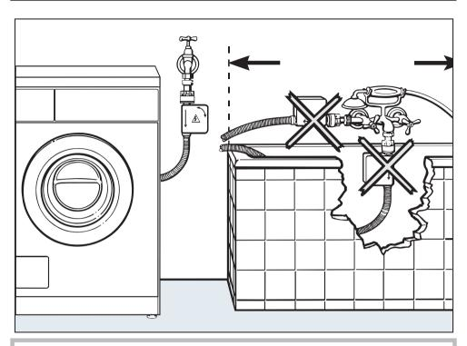
The plastic casing of the safety valve contains electrical components. The Waterproof system must only be connected to its own stopcock. It must not be connected to mixer taps or similar and must not be fitted in areas where there is the risk of water or other liquids reaching it.
