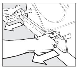
3 Withdraw the two bars together with the support plate.
